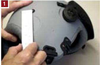
Locating the drilling hole
