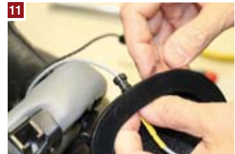
Drilling and routing of the wire (HGU-55 and ACS style)
