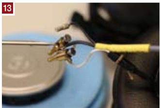
Place the original audio connector in to the hole located in helmet kit connector and secure the screw.
